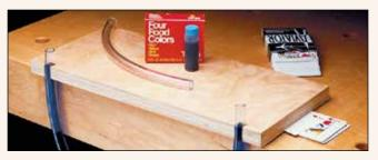
lower. Then simply shim under the side of the level where the water is highest until the water columns are equal. (I used playing cards for shims.) Now use the surface to check your level.
