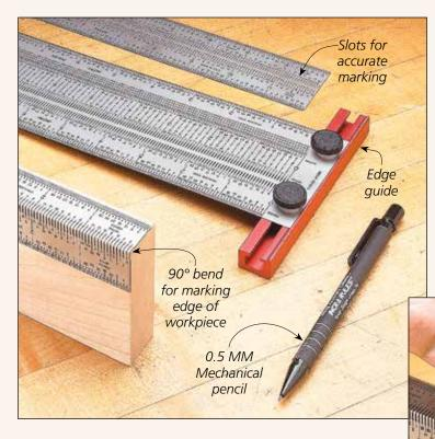
Another advantage of mechanical pencils is that they don't need sharpening. You simply advance the lead as it wears down. Inexpensive replacement leads are available once the original lead is used up. And like standard pencils, you can buy replacement leads in several
